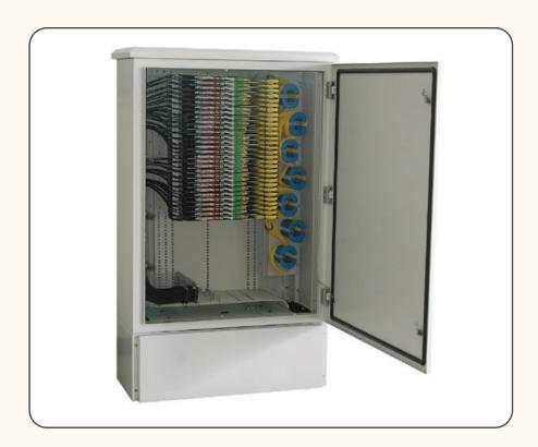
Suitable for use in the network where optical splitters are distributed. It offers optical cable stripping and a fixing assembly, optical splitter module, splicing module, and storage area, completes the functions of optical cable inlet fixing, fibre splicing and termination, optical splitter installation management, and coiling, storage, fixing, and splicing of single-fibre drop cables, and implements optical splitting and capacity expansion of optical lines.
